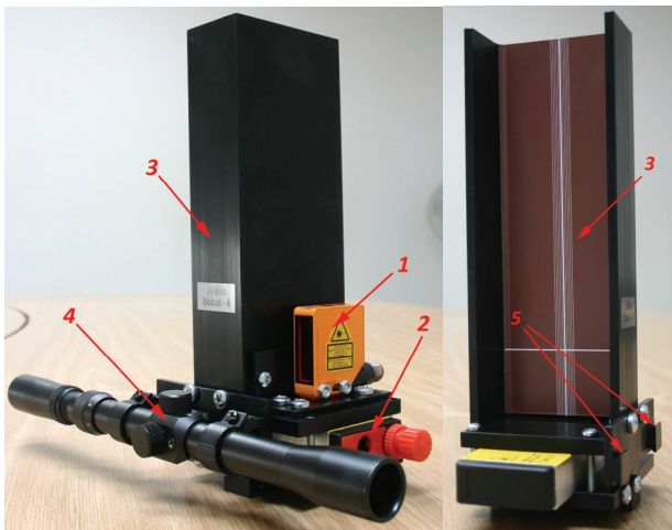
Fig. 2. Laser unit: 1 – laser sensor; 2 – laser level; 3 – aim board; 4 – telescopic sight; 5 – place for telescopic sight
