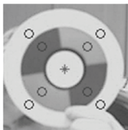
Fig. 4. The nine pixels which are used for marker recognition
