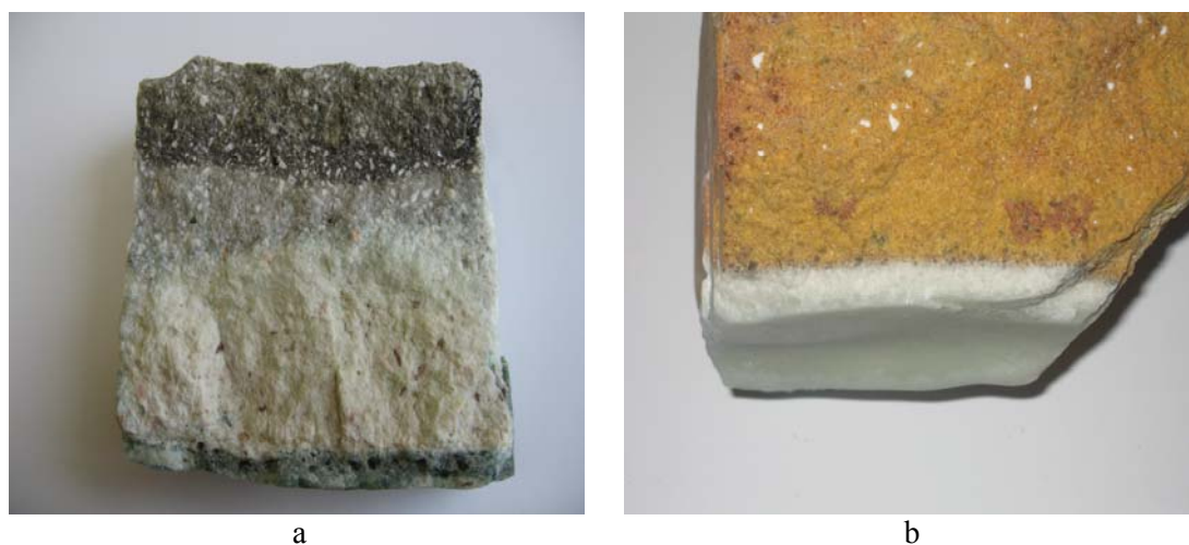
Fig.1. The photos of used dinas bricks: a) from the crown of container glass furnace; b) from the crown of electrovacuum glass furnace.
