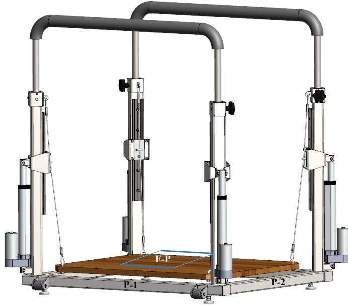
Figure 45. CAD rendering of the adaptive balance platform. The suspended board hangs on steel cables whose effective lengths are adjusted by four corner-mounted linear actuators to modulate suspension geometry and produce programmable multidirectional instability. A force platform (F-P) is located under the board, and frame-mounted proximity sensors (P-1, P-2) estimate board position in the horizontal plane (x and y coordinates) and quantify displacement. Adjustable safety handrails are integrated into the open aluminum frame. Labels: F-P - force platform; P-1/P-2 - proximity sensors
