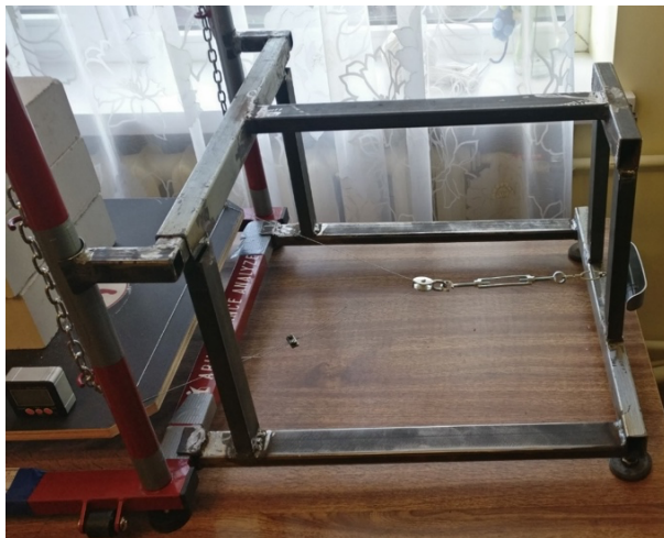
Figure 9. Static force–displacement test set-up. An auxiliary frame (1) supports a digital force transducer (2) that applies and measures horizontal force F . The board is pulled by a non-elastic cable (3) to impose anterior displacement d while load mass m is centred on the board. Force was recorded at 0.05 m displacement intervals. Labels: (1) auxiliary frame; (2) digital force transducer; (3) non-elastic cable
