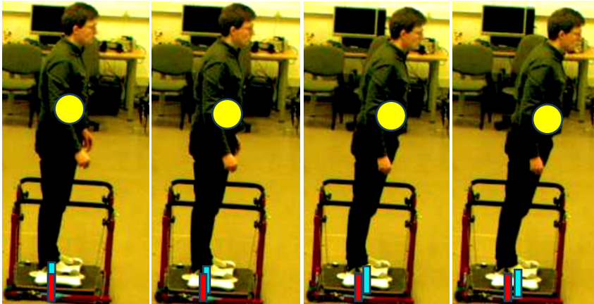
Figure 31. Experimental task. Start: vertical alignment of p-COM (yellow), BOS center – the platform board center (blue), and a fixed ground reference (red). The participant performs a controlled forward lean using ankle motion only. Two phases are shown: coupled – p-COM and BOS move together while the board tilts; uncoupled – once the board stops tilting (BOS no longer displaces), p-COM continues forward while BOS remains fixed. Left to right: initial alignment → coupled phase → uncoupled phase. The sequence illustrates the single permitted degree of freedom at the ankle
