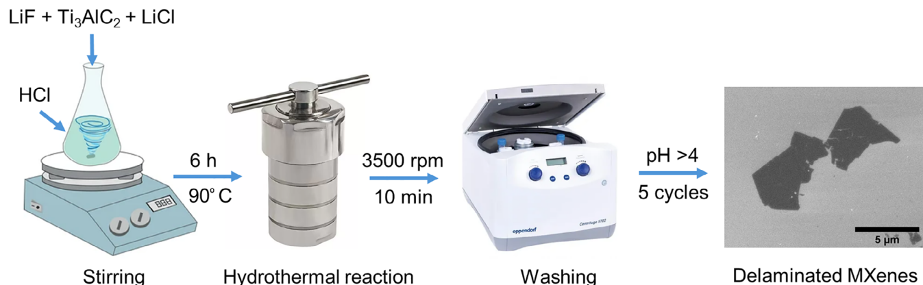
SCHEME 1 | Schematic illustration of \text{Ti}_3\text{C}_2\text{T}_x MXene synthesis from MAX phase precursor.
