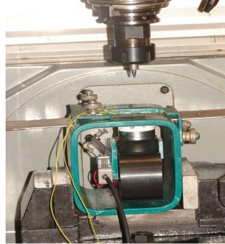
Fig. 3 Friction drilling experimental set up: a - overview; b - drilling device
