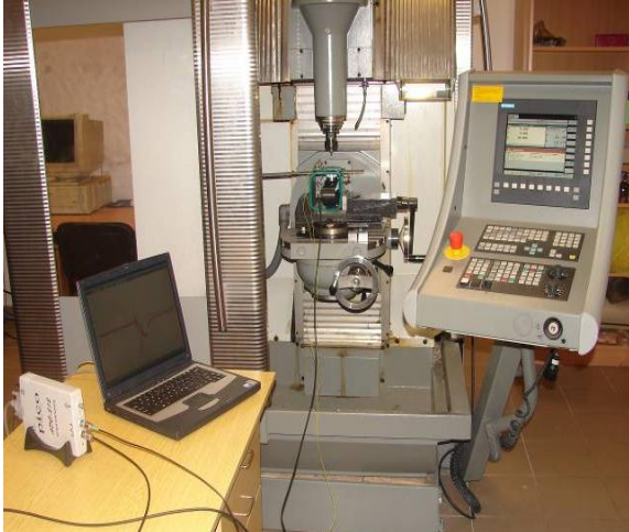
Fig. 3 Friction drilling experimental set up: a - overview; b - drilling device
