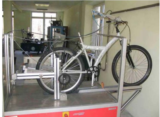
Fig. 2 Test facility for brake testing
