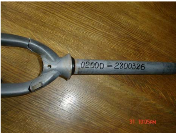
Fig. 7 The fork after 65057 cycles of testing with 600 N load
