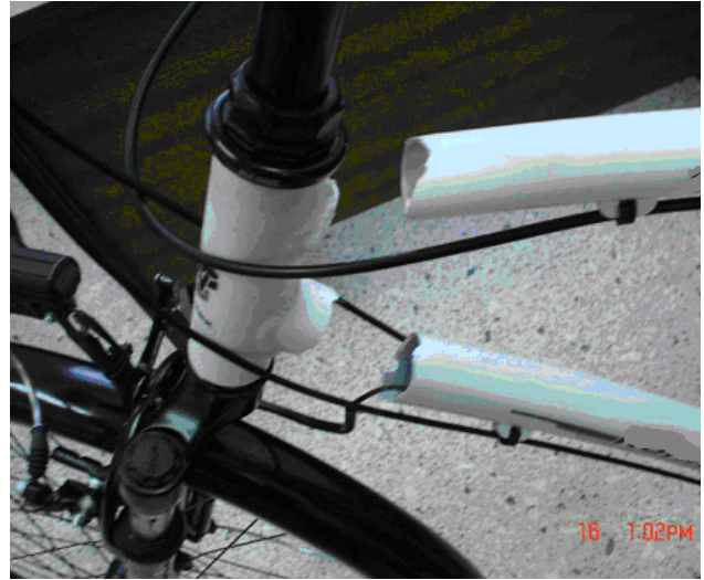
Fig. 8 Break of both frame tubes after riding of tourist bicycle distance of 230 km on stand with reels
