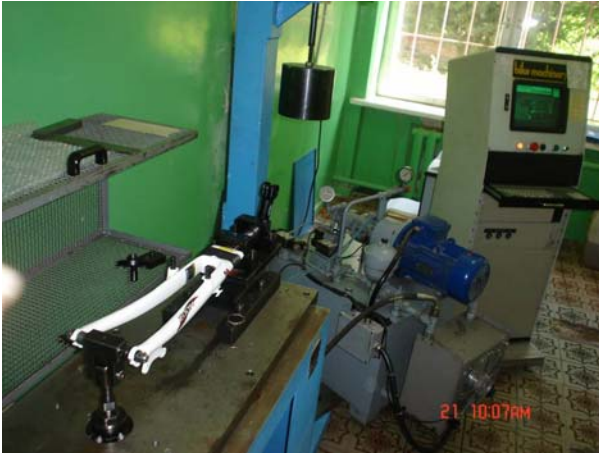
Fig. 6 The front fork on the testing-bench
