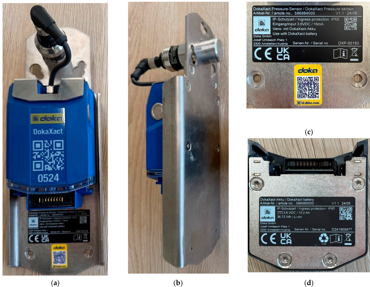
Figure 5. DokaXact measurement unit with integrated sensor connection (a) top view; (b) side view; (c) information label; (d) battery module.
