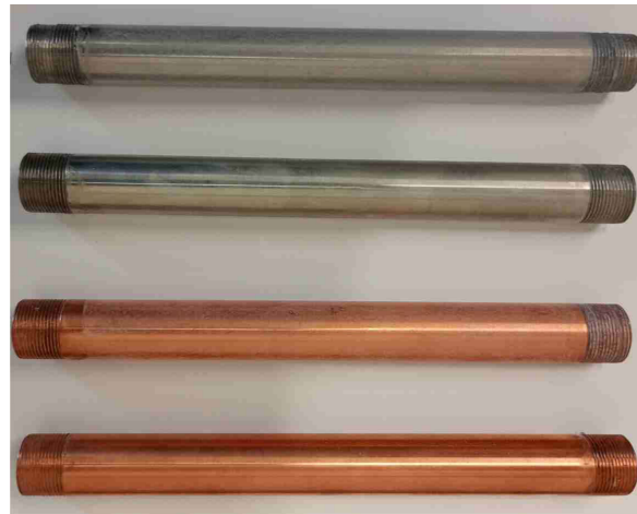
Figure 3. Representative views of the tested modified surfaces: ZnO and ZnO/PMHS coatings on copper and stainless-steel substrates, and the Al 2 O 3 coating on the steel substrate.
