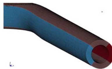
Fig. 5 Pipe elbow. Modelled with finite element consists of three zones: tension, neutral, and bended
