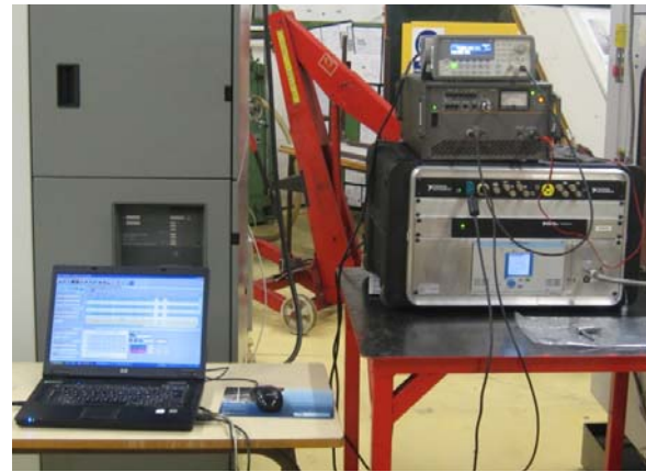
Fig. 6 Photo of measurement setup (Fig. 4) used for vibrational drilling experiments (high-frequency generator, power amplifier, KISTLER platform controller and power amplifier, computer)
