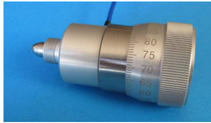
Fig. 11. Micrometric screw with piezo-adjustment
