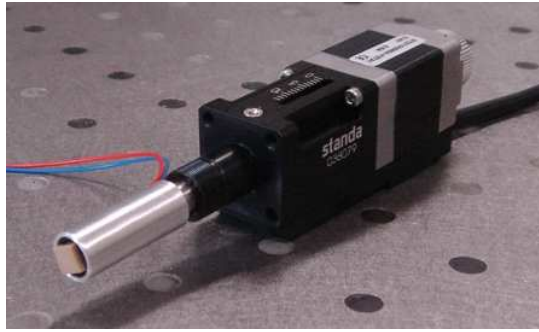
Fig. 3. Piezoelectric actuator mounted on motorized actuator
