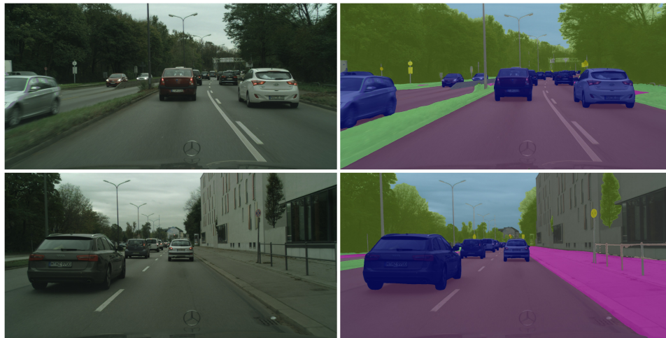
Figure 3: Example images with original one on the left, and segmented result on the right.
