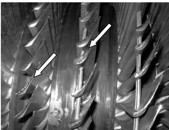
Fig. 7 Traces of rubbing between rotor and stator blades: a - traces of rubbing between rotor and blades of stator, b - traces on rotor blades left by broken blades
