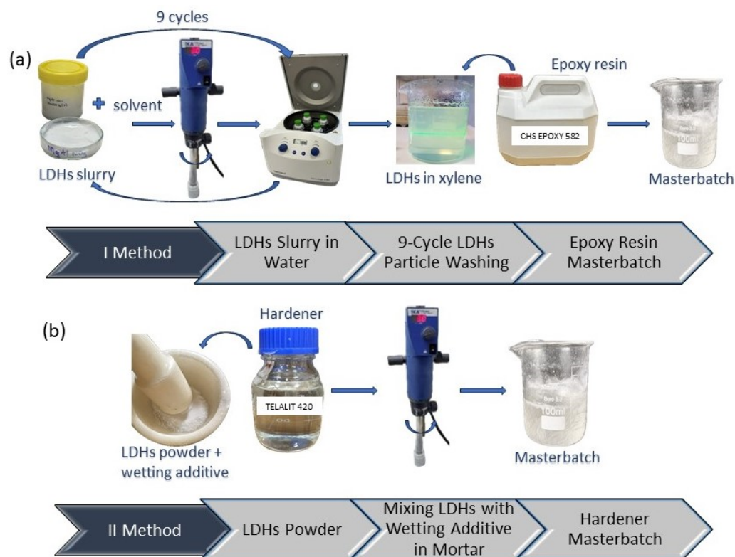
Figure 1. LDH masterbatch preparation methods based on the utilisation of: LDH slurry in water and gradual substitution for organic solvents (a); LDH powder with wetting additive (b).
