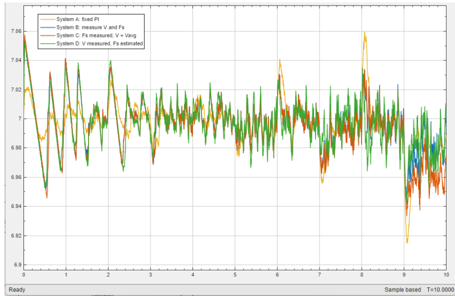
Fig. 30. Added noise at \sigma_{CH} = 1e^{-8}, \text{mmol/L} (X axis - Time(h), Y axis - pH)
