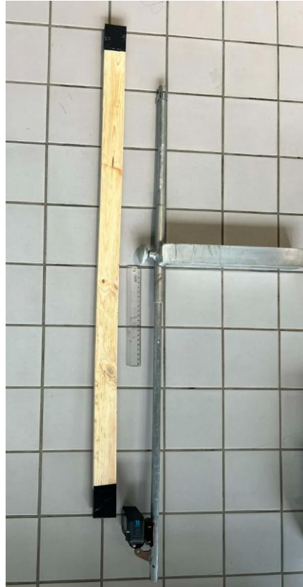
Fig. 25. Calibration stick used for spatial scaling and plane alignment
