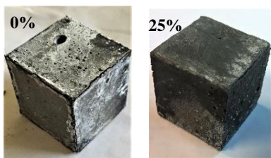
Fig. 10. Optical photos of cement samples (30×30×30 mm) with 0 and 25 wt.% of the AFA additive after 9 months of maintenance in 5% Na 2 SO 4
