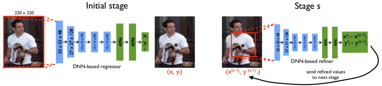
Fig. 1. Schematic view of the DNN-based pose regression and refinement [6]
