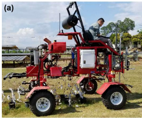
Figure 2. Lab-based hyperspectral Collection System [8]
