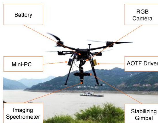
Figure 3. UAV-Based Hyperspectral Imaging System [13]
