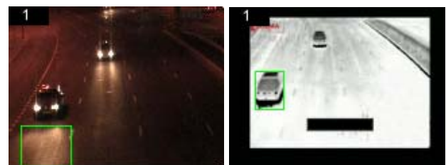
Fig. 10. Vehicle flow recognition at night
