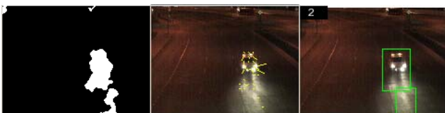
Fig. 4. Vehicle flow recognition at night
