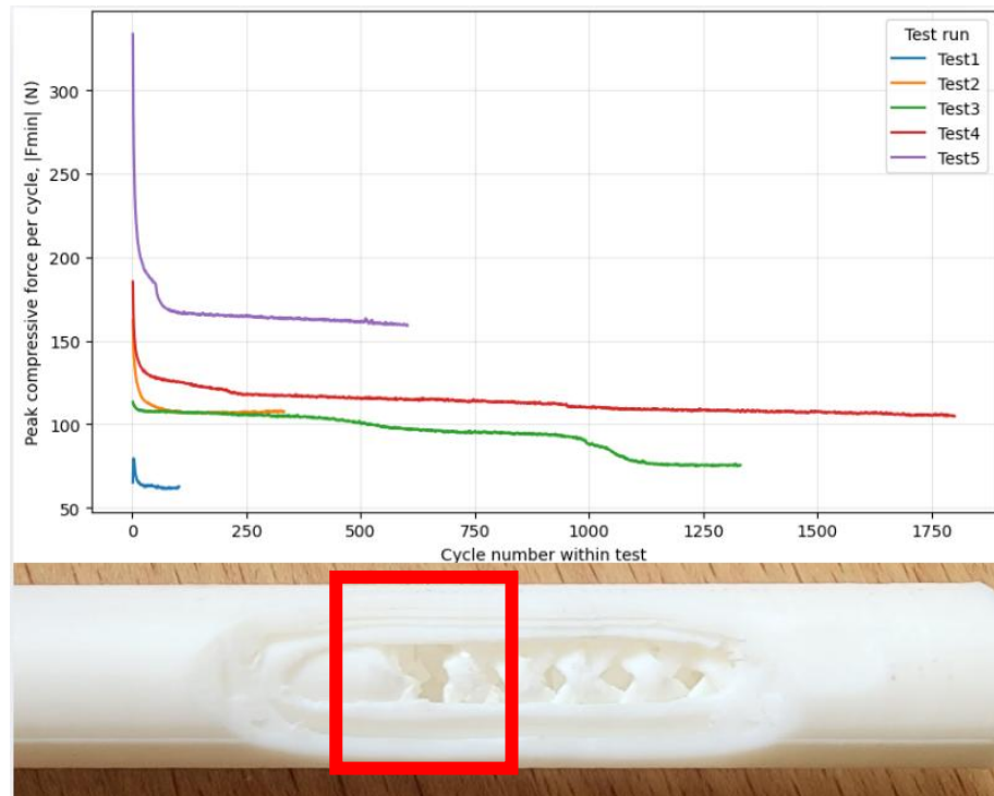
Fig. 19. Results of the experimental cyclic testing with the damaged cross-section opened view
