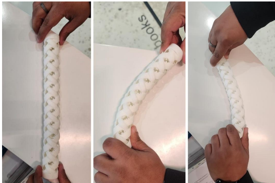
Fig. 5. Buckling of structure
