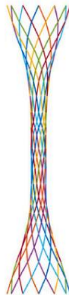
Fig. 3. Necking of CFT [27]
