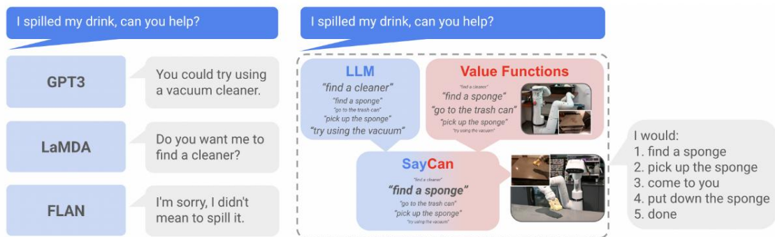
Fig. 7. Example of how the SayCan model works using a natural language query to generate instructions that are appropriate for the bot.
