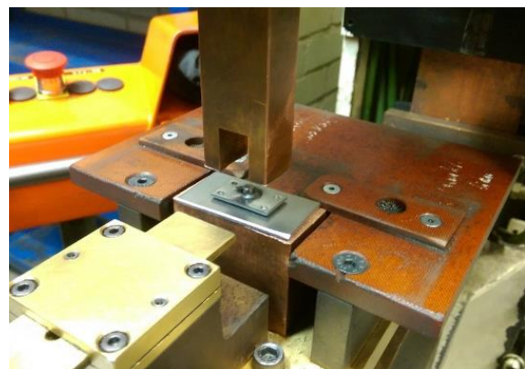
Fig. 2 Contact nuts welding equipment
