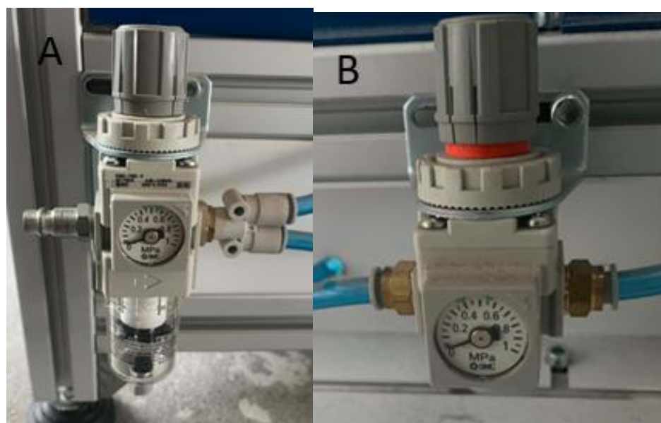
Fig. 24. A – Compressed Air Filter; B – Compressed Air Regulator
