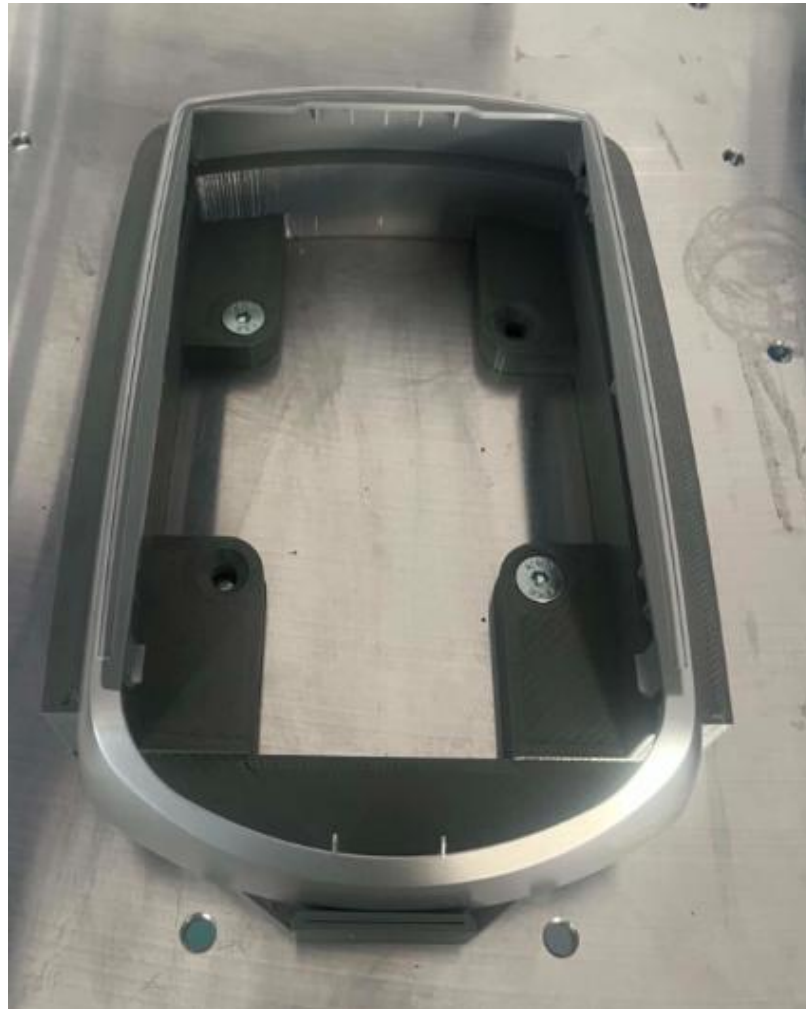
Fig. 22. Holding Component Printed and Mounted
