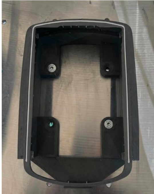
Fig. 34. Result of the Dispensing, with a Successfully Extruded Line
