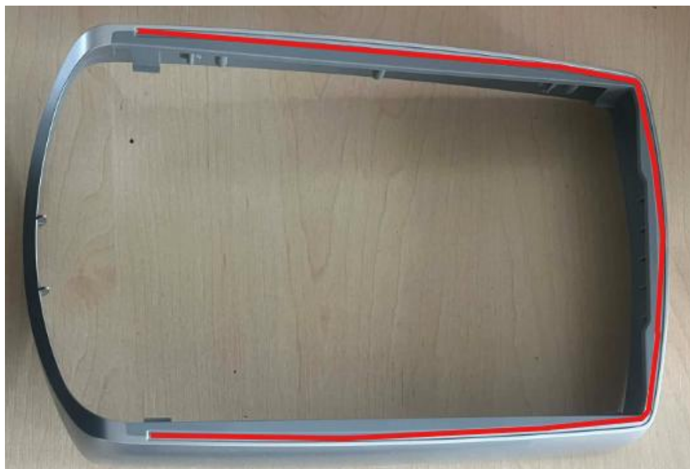
Fig. 8. Part Provided by Company X, Red Lines Mark the Area Where the Adhesive Should Be Dispensed
