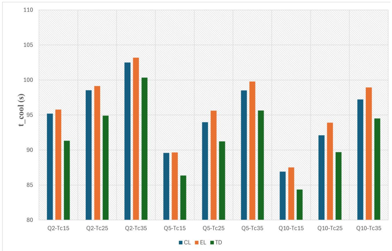
Fig. 12. Comparison of cooling time ( t_{cool} ) for circular, elliptical and teardrop CCC profiles under matched coolant flow rate and coolant temperature conditions
