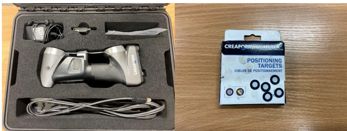
Fig. 6. Used equipment for 3D scanning (HandySCAN 700 and position targets)
