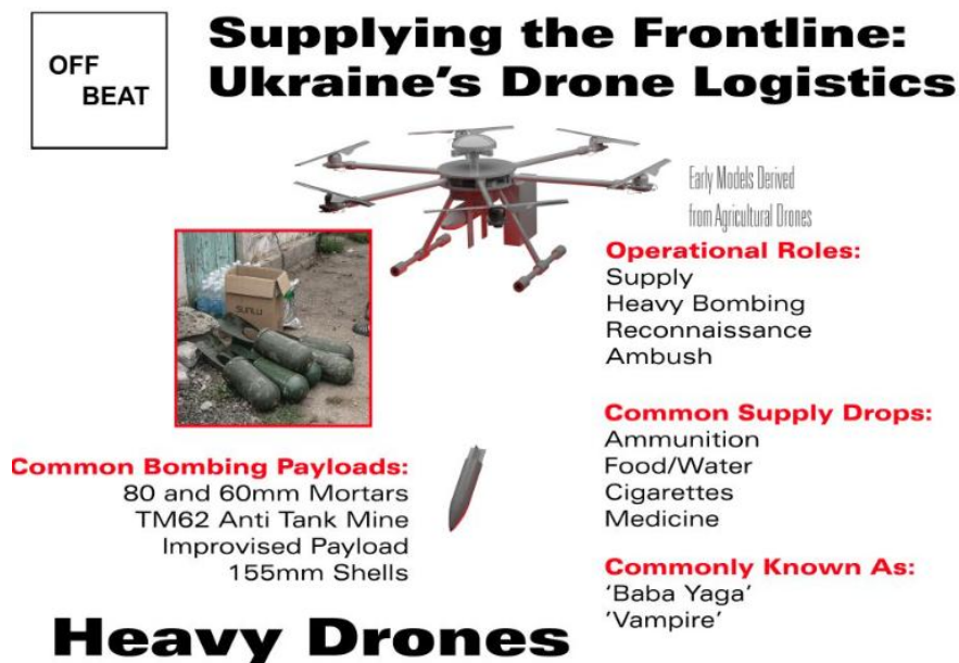
Fig. 1. "Baba Yaga" Military Logistics Drone With List of Common Uses [4]
