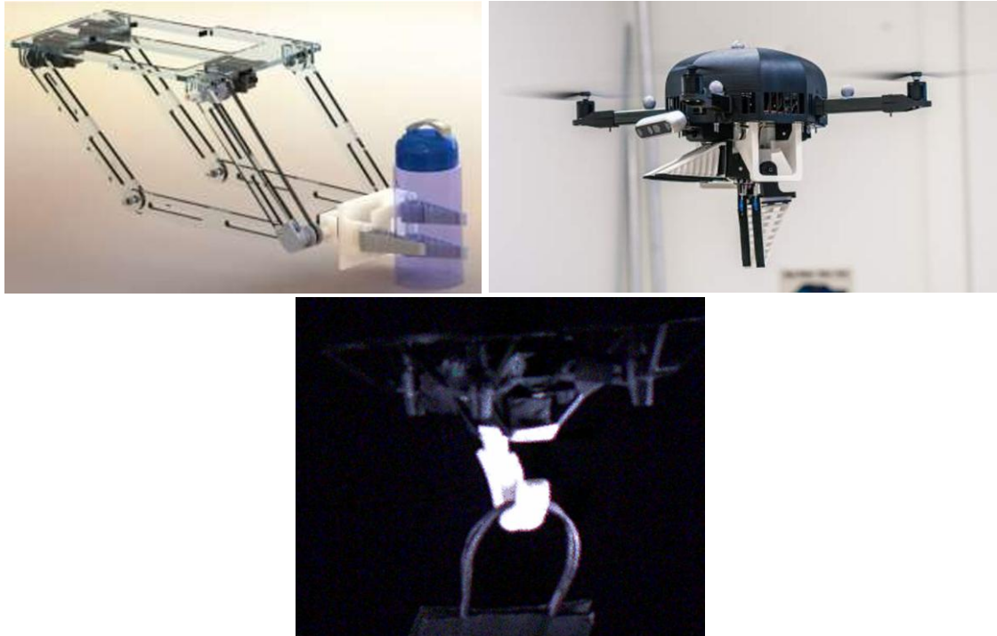
Fig. 12. Left: Automatic Item Pick-Up Gripper [27]. Right: RAPTOR Pick-Up Gripper [28]. Bottom: Hook Type Gripper [29]
