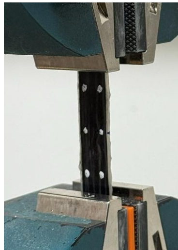
Fig. 22. Tensile specimen placed in the grips
