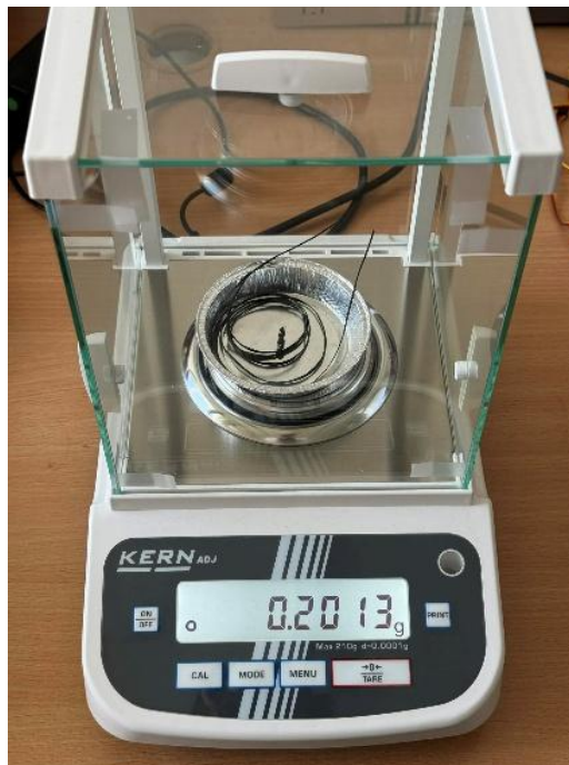
Fig. 12. Fibre tow weighing using analytical scales
