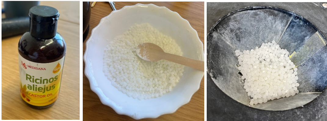
Fig. 22. Castor oil (left), mixed material (middle), mixed material in extruder (right)
