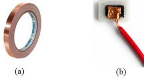
Fig. 21. (a) Copper Adhesive Tape (b) wire attachment using the tape
