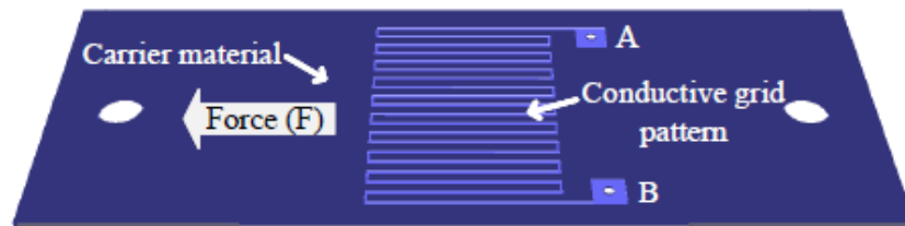
Fig. 9. Components of the FDM-printed strain gauge showing carrier material, conductive grid pattern, and contact pads [13]
