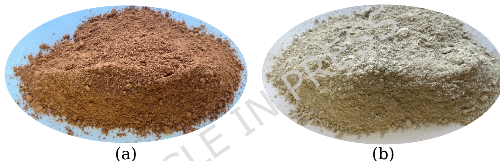
Fig. 1. Images of the precursor materials: (a) - CBW, (b) - MKW.
