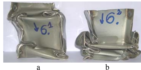
Fig. 8 Specimens after the dynamical crushing: a – with good spot-welding; b – with collapsed spot-welding in two places
