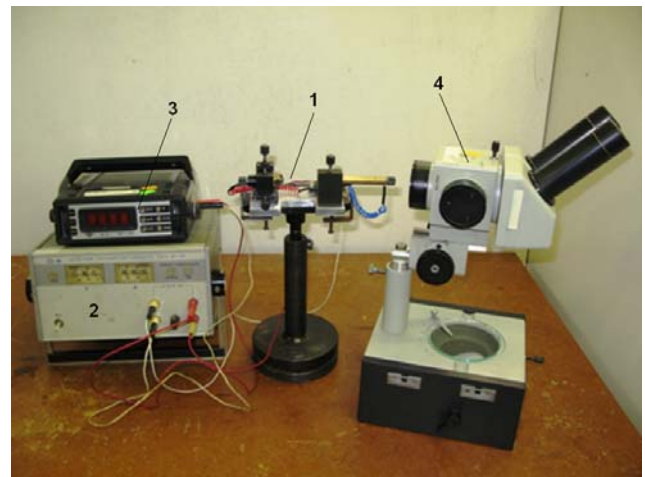
Fig. 2 Technological set-up for the tungsten wire tip sharpening operation: 1 – etching manipulator; 2 – DC source B5-46; 3 – parameter control device B7-35; 4 – microscope MBC-9
