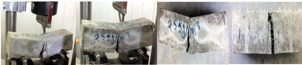
Figure 7. Concrete samples after final bending result.
