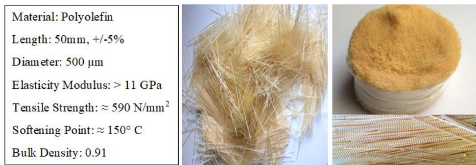
Figure 1. Properties of polyolefin macro fibers.
