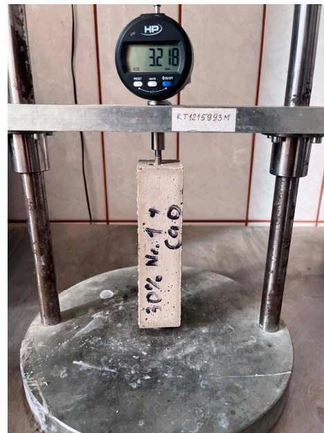
Figure 7. The shrinkage measurement setup.
