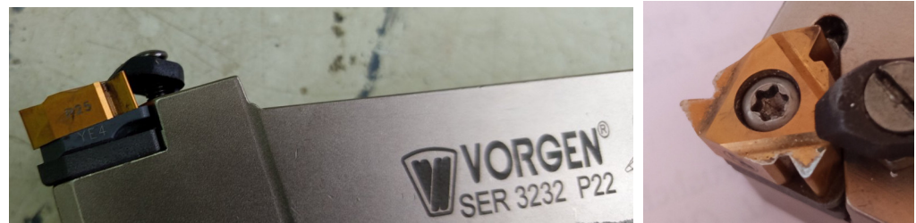
Figure 22. Threading cutting tool with two shims: side view and top view of the thread cutting insert.
