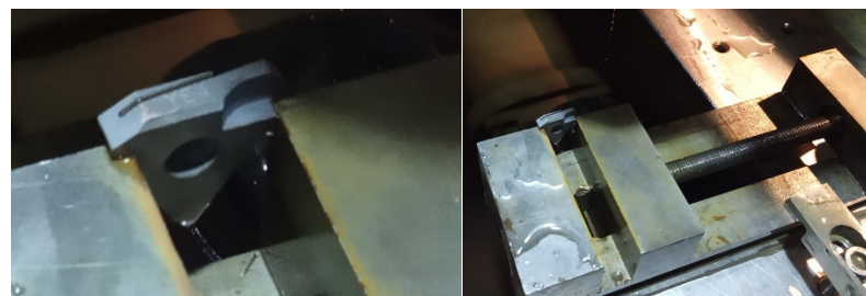
Figure 23. Electro-spark discharge machining of the backing shim.
