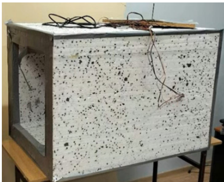
Figure 3. Heating box with convection heat source (Poland, Gliwice).
