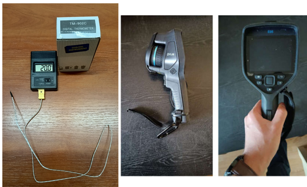
Figure 2. On the (left), the TM902C meter with a probe; on the (right), the Flir E95 camera [75].
