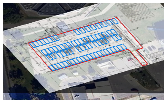
Figure 1. Map overlaying with QGIS: (red bounding) parking boundaries, (blue bounding) boundaries of each parking space.
