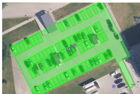
Figure 2. Vehicle detection and parking space segmentation overlay.
