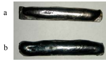
Fig. 4 Single - pass welded layers: a - welded under glass powder, b - under standard AMS1 flux
