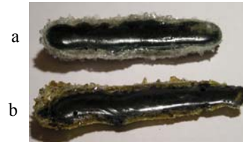
Fig. 5 Hardened slag removed from the layers welded under glass powder (a) and under standard AMS1 flux (b)
