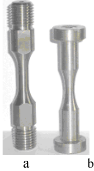
Fig. 1 Specimens used in the investigation: a - cylindrical, b - corset type
