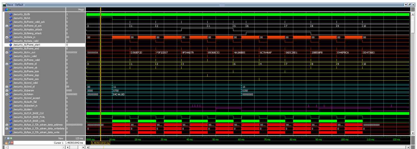
Figure 3. Timing simulation of the integrated hardware security modules summarized in Table 3. The waveform illustrates the concurrent operation of multiple protection mechanisms within a unified testbench. White signals correspond to the replay/timing detector, orange to the CRC-32 integrity module, yellow to the frame counter monitor, cyan to the command authentication module, and magenta to the traffic anomaly monitor. Red traces represent SDRAM interface activity, while green signals denote camera synchronization signals.
