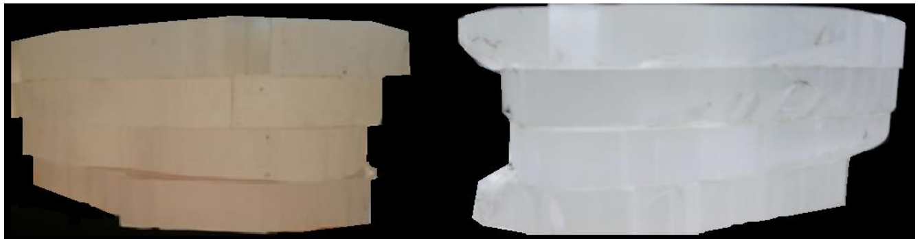
Figure 16. Result of polishing process; on the left – before polishing; on the right – after polishing
