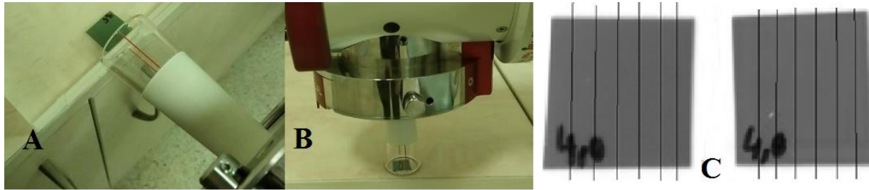
Figure 21. GAFchromic film calibration process; A – film irradiated in a 90° angle, B – film irradiated at a 0° angle, C – film fragmentation for analysis with irradiation dose of 4 Gy, left – irradiated in condition A, right – in condition B
