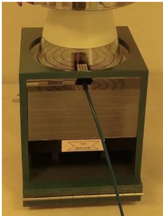
Fig 7. Ionization chamber PTW 23342 and phantom T2962 system used as reference system for measurements.
