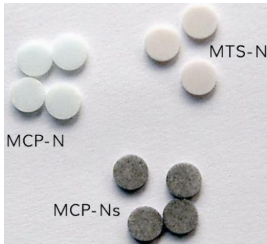
Fig 3. Different pellets of LiF based TLDs: MTS-N is LiF: Mg,Ti (TLD) MCP-N and MCP-Ns is LiF: Mg, Cu, P [30]
