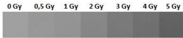
Fig.14. GafChromic EBT2 film irradiated with different ionizing radiation doses
