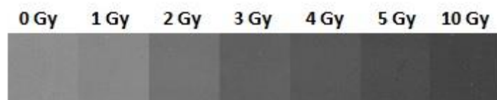
Fig.13. GafChromic RTQA 2 film irradiated with different ionizing radiation doses
