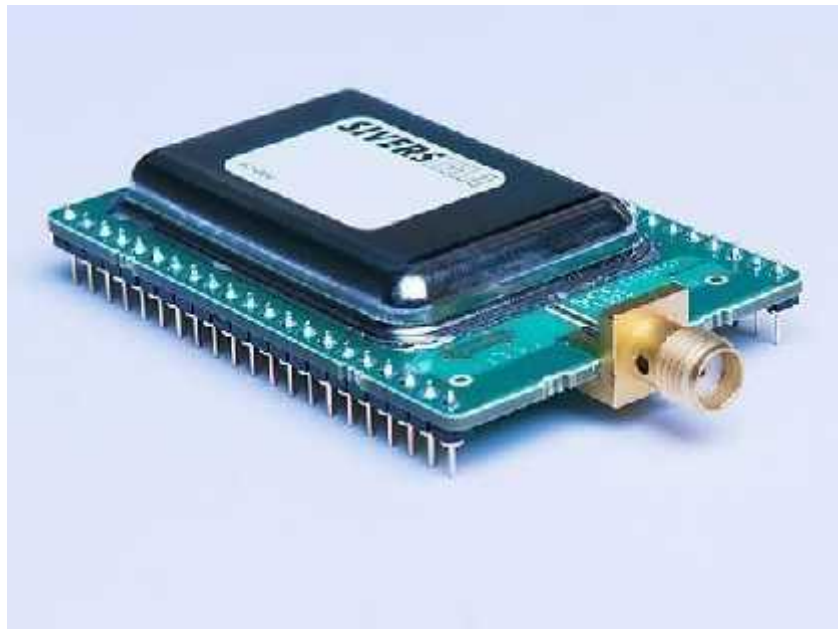
Figure 2. 3 Radar Sensor involved in the FMCW radar system. [21]
