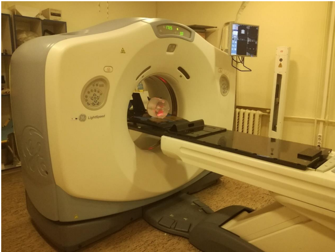
Fig. 2.10.1 Couch with combiboard set up for CT scanning, for calculation of attenuation in lung area with Eclipse™
