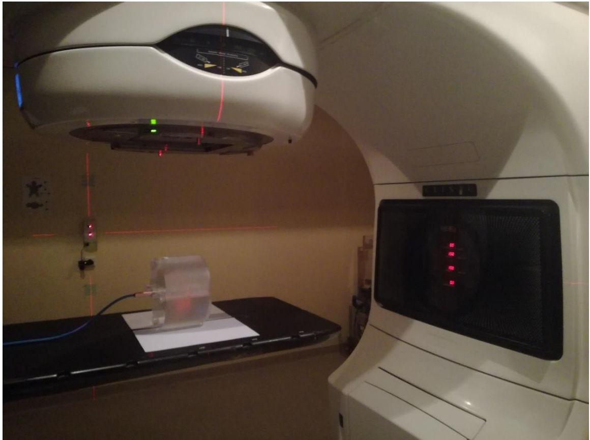
Fig. 2.9.1 Varian Exact IGRT couch top attenuation evaluation set up, lasers passes through phantom geometrical centre
