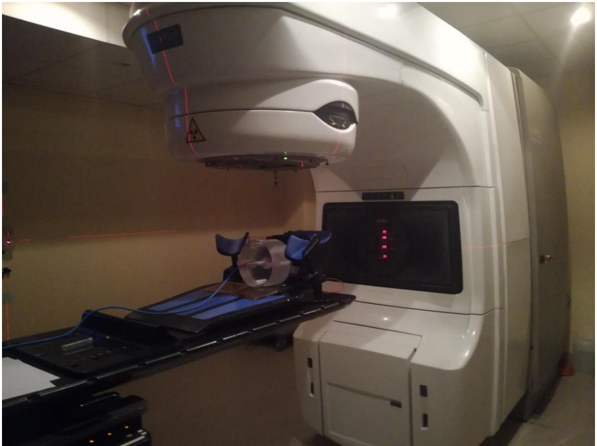
Fig. 2.9.3 Couch with combiboard attenuation evaluation set up for lymph nodes, oesophagus location, lasers passes through phantom geometrical centre
