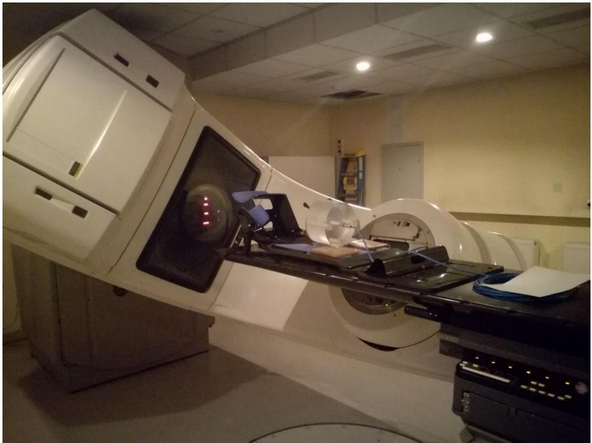
Fig. 2.9.2 Couch with combiboard attenuation evaluation set up for lung area, oblique beam angle
