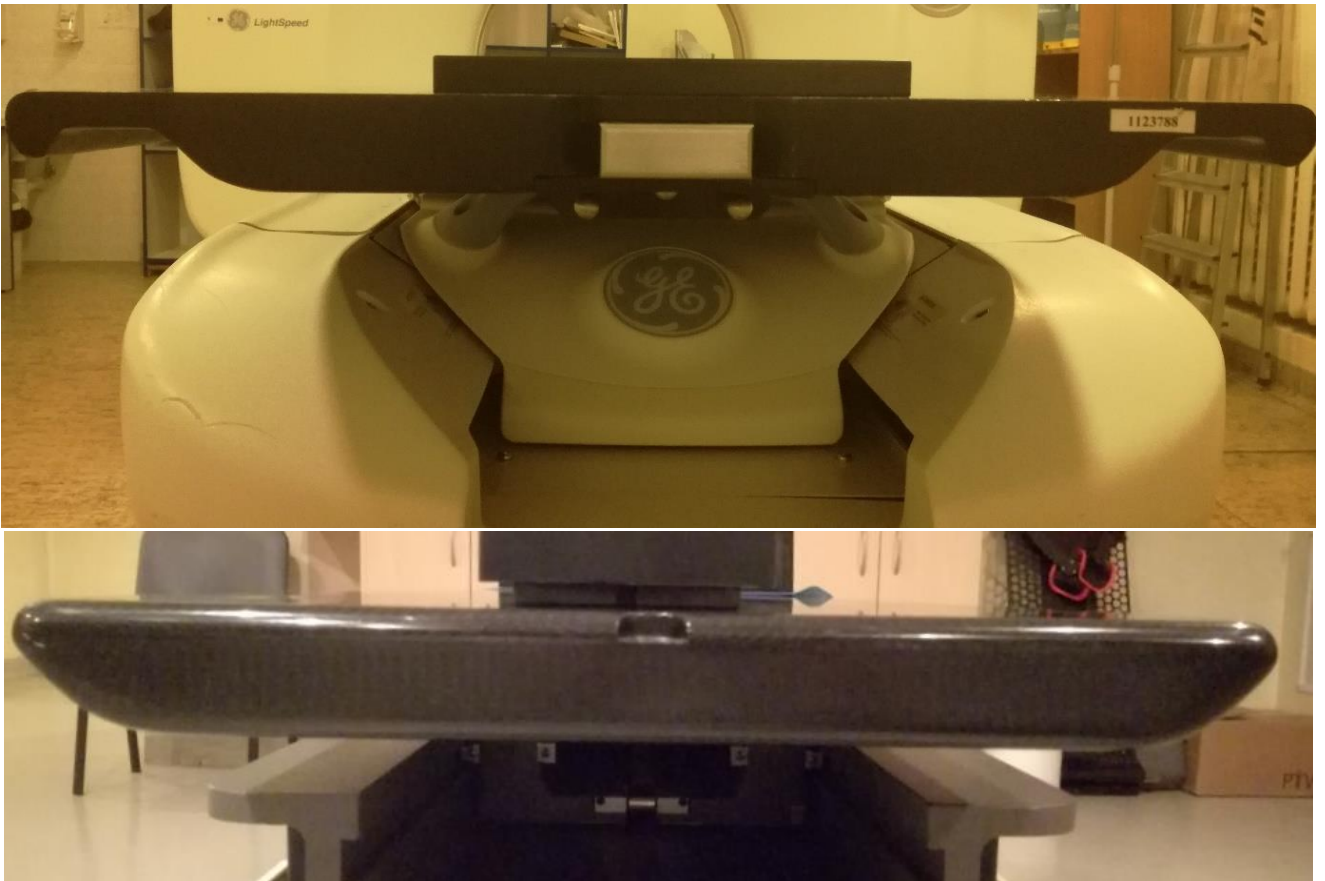
Fig. 3.3.5 Top - Diacor CT overlay profile and bottom - Varian Exact IGRT couch top profile
