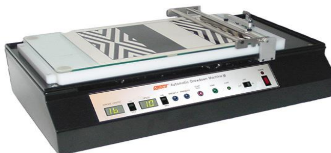
Figure 22. Mayer rod machine for laboratory [46]
