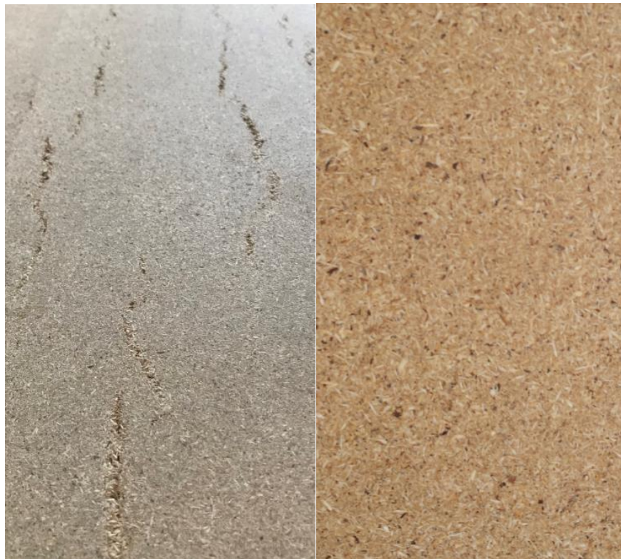
Fig. 18 a) Surface of particleboard after intermediate belt failure b) Surface of A quality particleboard
